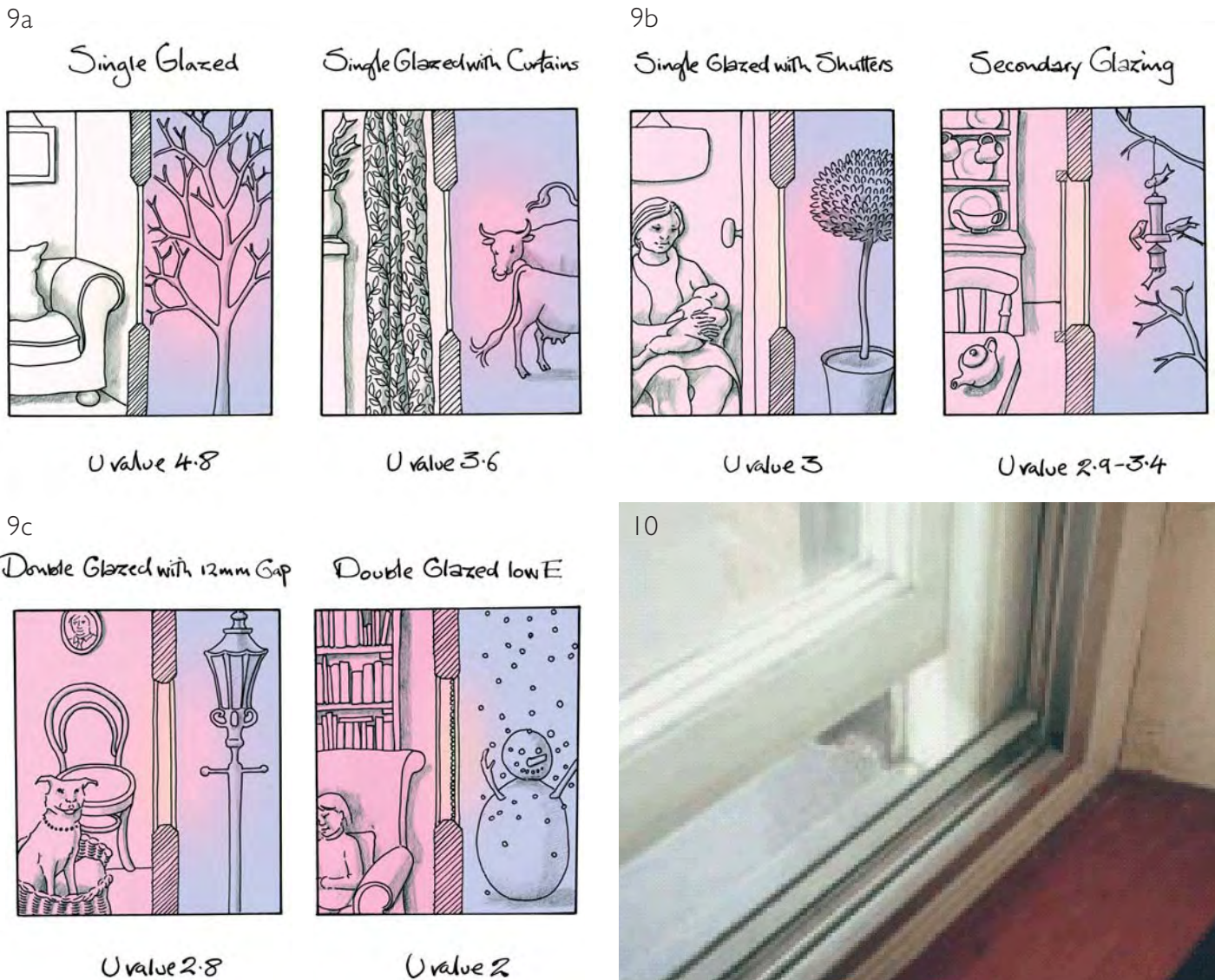
9a+9B+9c Indicative U values (W/m 2 deg C) for vertical glazing, with wooden or PVCu frames 10 Secondary glazing reduces heat loss while retaining the existing window and its external appearance. (Photograph courtesy of English Heritage)
